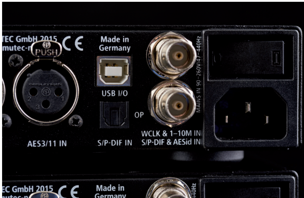
The right half of the rear panel with clock and digital inputs in detail
