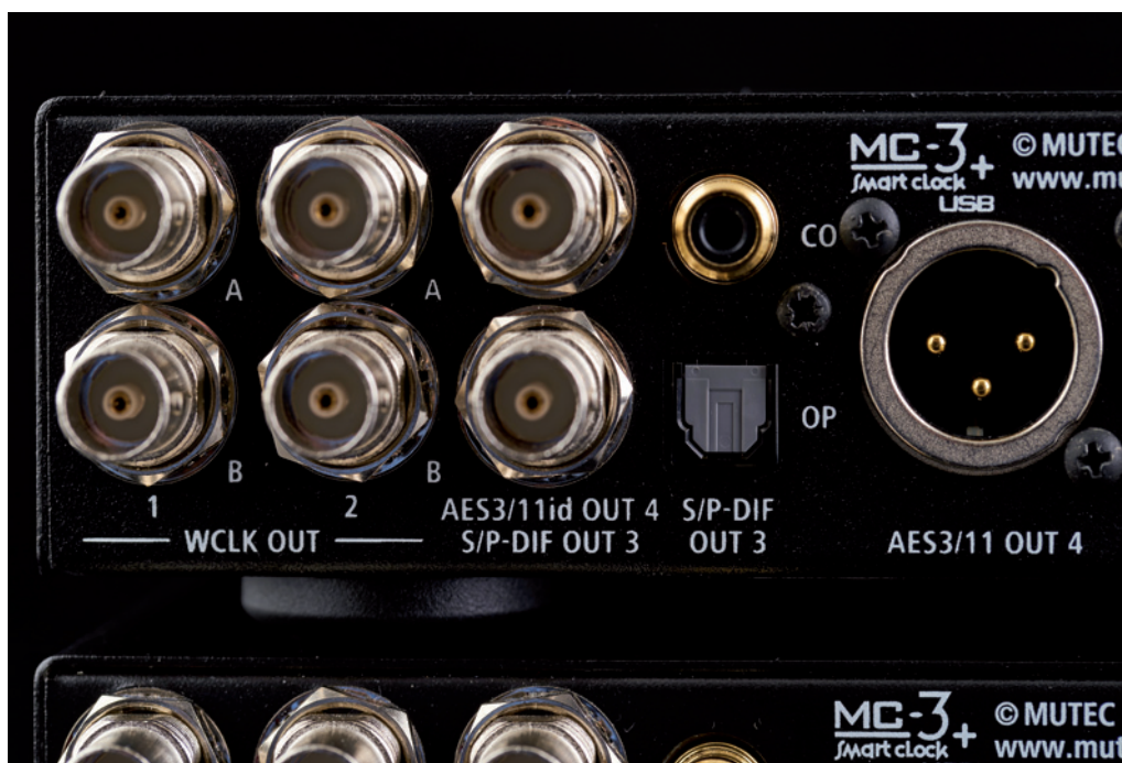
The left half of the rear panel with the four clock and the five digital audio outputs in detail
